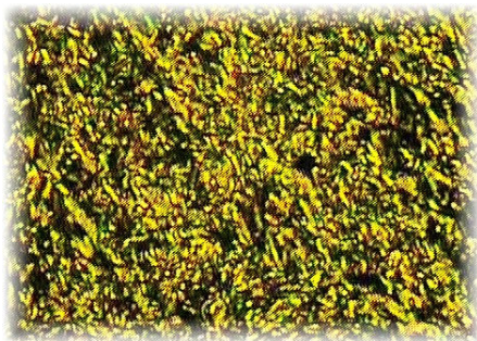
Fig. 2. Paramorphic mosaic texture of the smectic A phase, at heating from the solid state. Crossed polarizers, 136 ^{\circ}\text{C} ( \times 100 ).
