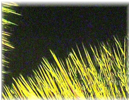
Fig. 3. Growth of the smectic A phase, from the isotropic phase, at 138 ^{\circ}\text{C} . Crossed polarizers, ( \times 100 ).
