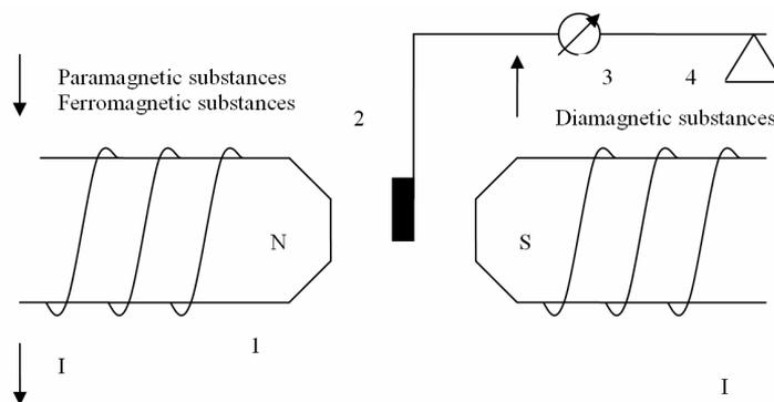
**Fig. 1** Principle scheme of Faraday method for magnetic susceptibility determination.
