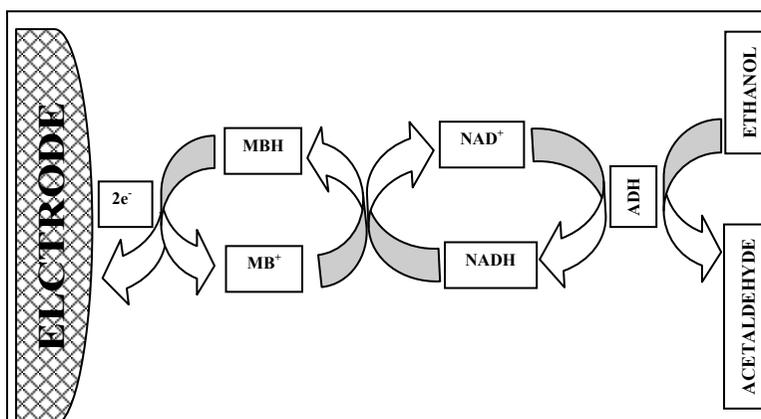
Fig. 2. Schematic representation of the mechanism of response of mediated ethanol biosensor
