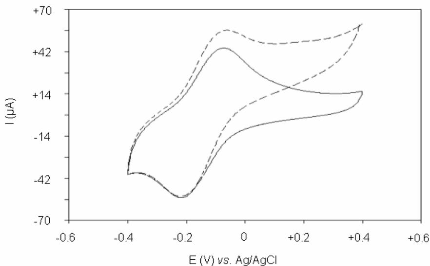
**Fig. 1.** Cyclic voltammograms at poly(MB) electrodes in the absence (—) and the presence (----) of  $5 \cdot 10^{-3} \text{ mol.L}^{-1}$  NADH.
