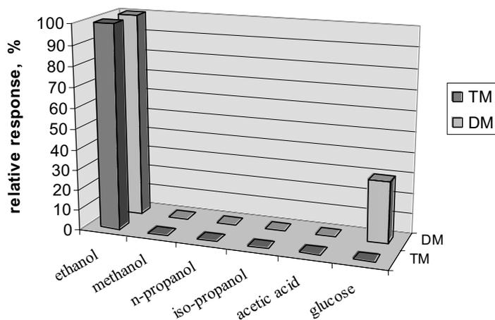
Fig. 4. Selectivity of the microbial biosensor for ethanol. (10 mM, 25°C, pH=7).
