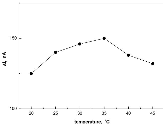
Fig. 2. *Effect of temperature on biosensor response (pH=7.00, ethanol 1 mM). Each point represents the average of 3 determinations.*
