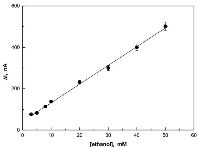
Fig. 3. Biosensor calibration curve (steady state, temperature  $25^{\circ}C$ ,  $pH=7.00$ ).
