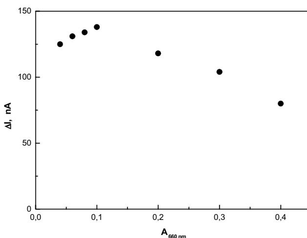
Fig. 1: *Optimisation of yeast cell concentration (temperature 25°C, pH=7.00, ethanol 10 mM). Each point represents the average of 3 determinations.*
