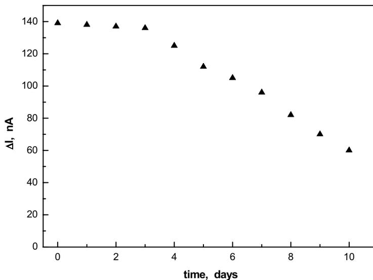
Fig. 5. Biosensor stability (temperature 25 °C, pH=7.00, ethanol 10 mM).
